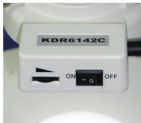
Dimmer integrated in lighting module
